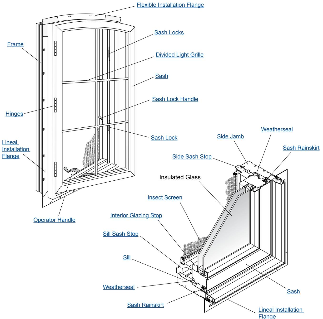
**Complementary Clad Casement Window Unit Parts - Standard Casements**
